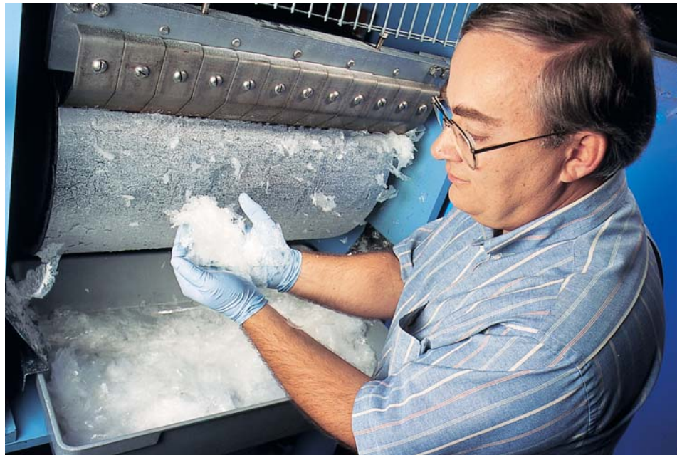
Chemist Fred Felker produces Fantesk flakes using a drum-drying process.
