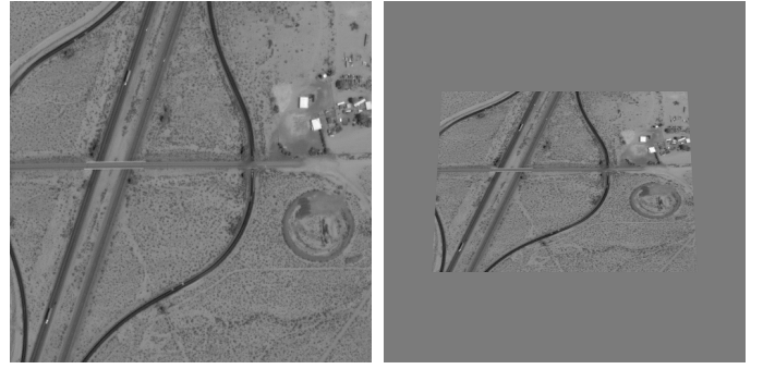
Fig. 10. Nadir and off-nadir image at 45^\circ simulated using a projective transform with an orbital height of 575 km.
