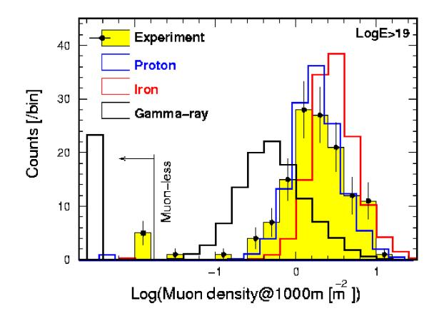
Shielded scintillators measure the muon flux.  $\rightarrow$  Primaries are mostly hadronic @ E>10<sup>19</sup>eV
