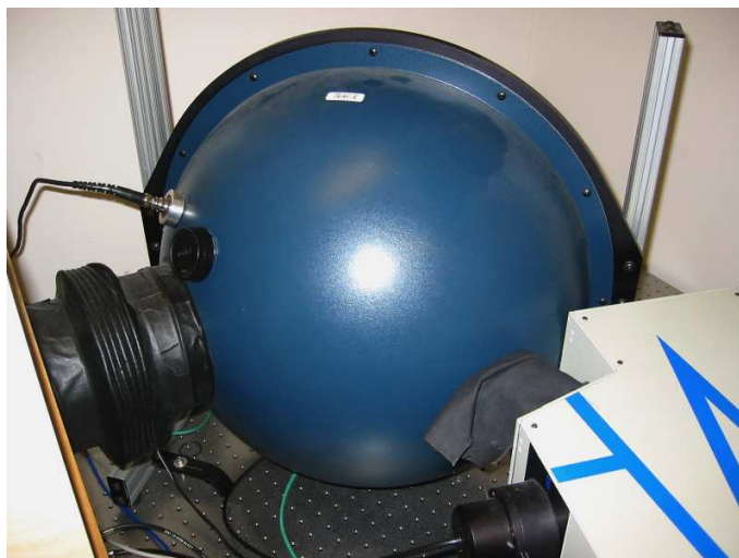
Figure 4.8: Shows the 20 inch integrating sphere. The 90° angle in the setup was employed for reasons of limited lab space.
