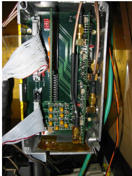
Figure 4.11: Infrared Labs ND-8 dewar. The dewar entrance port can be seen on the right. The feedthrough for the CCD signals is hidden behind the electronics box. A pneumatic actuator with mechanical feedthrough allows to move a x ray ^{55}\text{Fe} source in front of the CCD.
