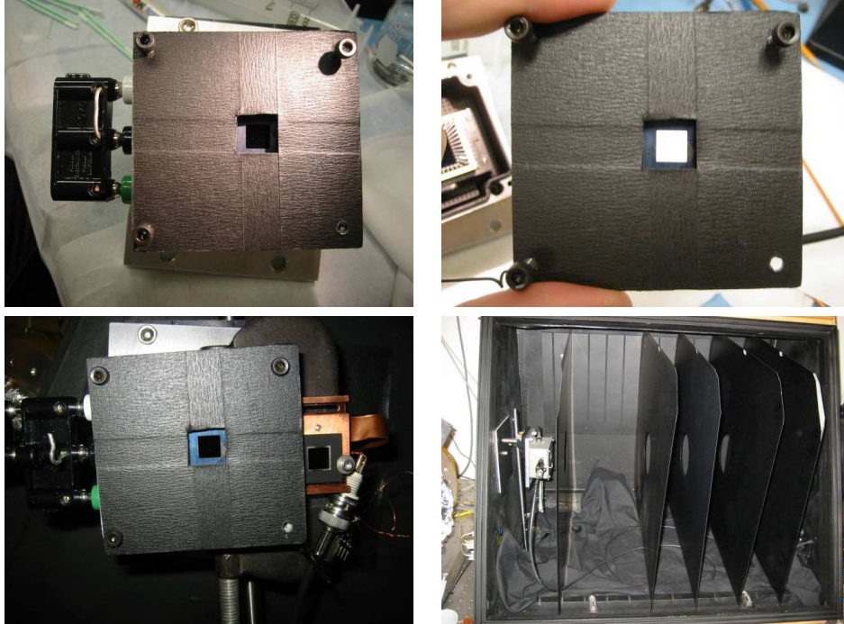
Figure 8.13: A 9 mm x 9 mm mask which was placed in front of the CCD. The remainder of the CCD was masked with black tape. The CCD and the photodiode were mounted next to each other close to the back wall of the dark box.
