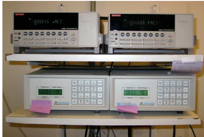
Figure 4.14: Two Keithley 6485 picoammeters measure the photocurrent of either the two calibrated photodiodes or of one calibrated photodiode and the sphere diode. The later setup allows light level adjustment without exposing the CCD to light and therefore without saturating the CCD.
