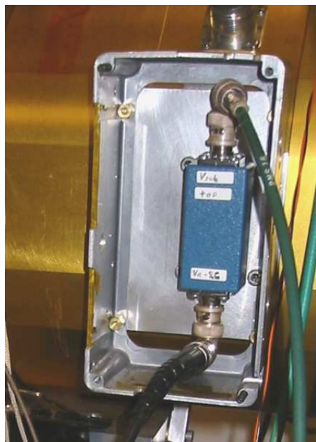
Figure 4.16: Adapter to operate the CCD in the photodiode mode.
