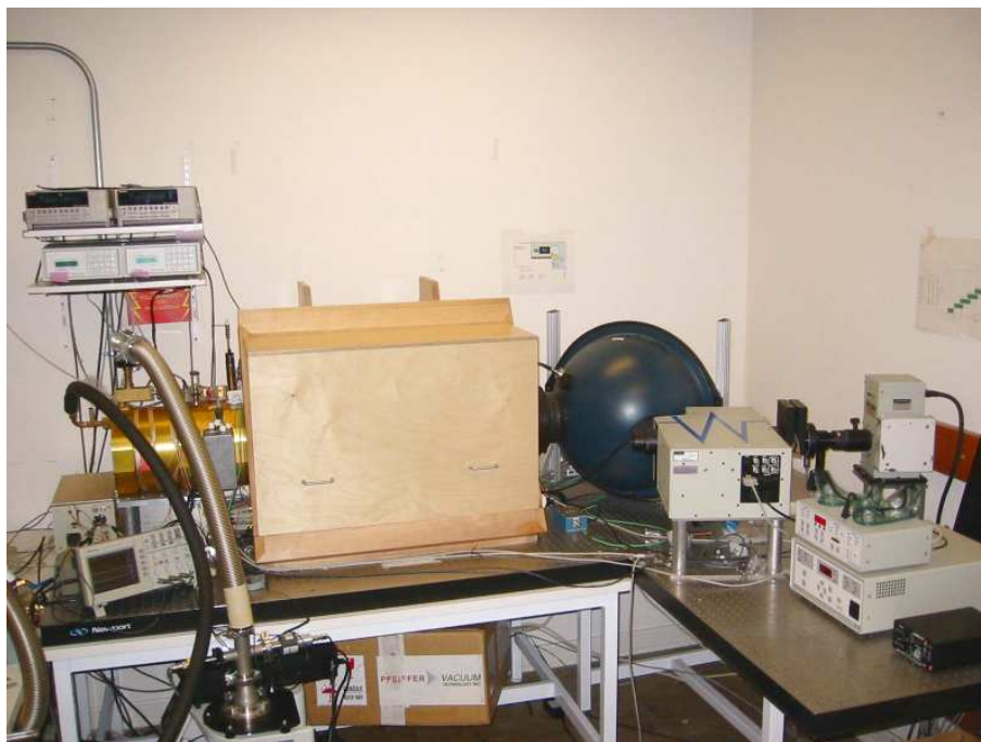
Figure 4.2: Overview of the QE setup. On the right one can see the light source and the monochromator. The monochromator feeds into the blue 20 inch integrating sphere. The sphere is attached to a 80 cm long dark box. The goldler dewar on the left holds the CCD and two temperature controlled photodiodes.
