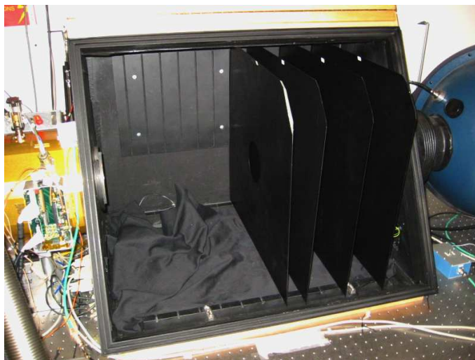
Figure 4.9: The inside of the 80 cm dark box.
