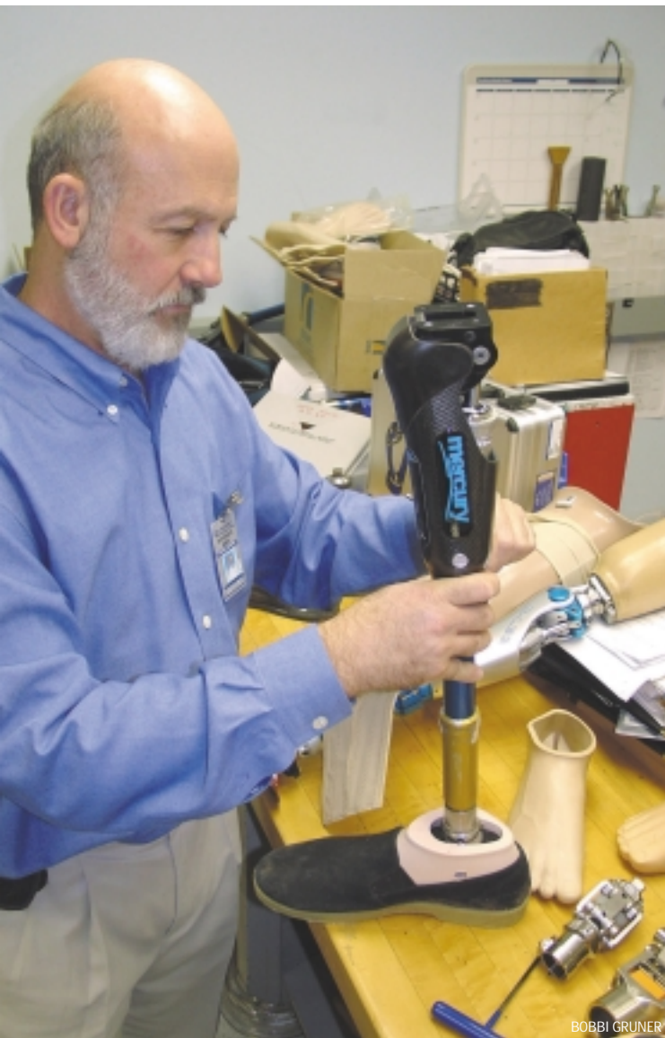
Prosthetist Mark Benveniste assembles a prosthetic leg using a hydraulic Mercury knee system at the Michael E. DeBakey VA Medical Center in Houston. The hydraulic knee allows users to ambulate at varying speeds and is frequently used as a back-up to the computerized C-Legs.
