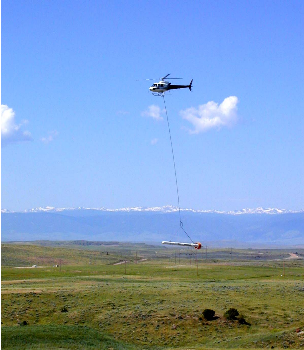
Figure 2 Helicopter electromagnetic survey of coalbed methane field in the Powder River Basin in Wyoming
