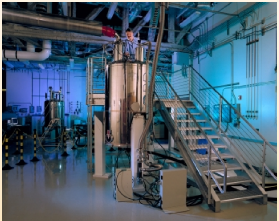
An 800 MHz nuclear magnetic resonance spectrometer in the William R. Wiley Environmental Molecular Science Laboratory is one of more than 15 NMRs available to help determine the chemistry of feedstocks or products.
