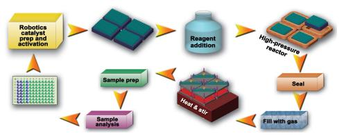
The Combinatorial Catalyst Laboratory (Combicat) is an integrated system for high-throughput catalyst experimentation at near-processing conditions, as can be seen in this schematic. This combination of high-throughput and processing conditions is unmatched at universities or other national laboratories.
