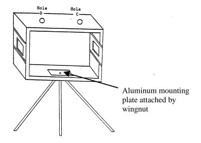
Figure 1 test stand attached to tripod
