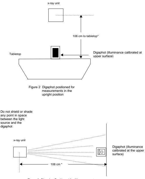
Figure 3 Digaphot Positioned for Measurement in the Horizontal Position
