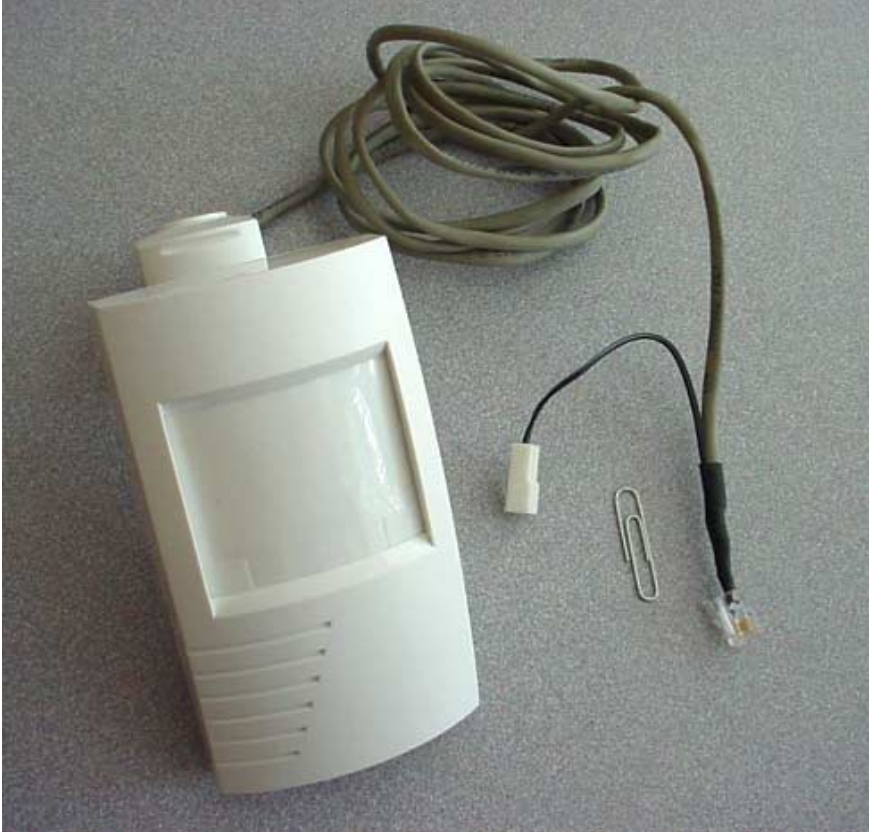
Figure 2. Prototype ceiling-mounted multisensor designed to measure desktop illuminance, temperature and occupancy. This multisensor is designed to be either ceiling- or wall-mounted. It measures the three key environmental variables and outputs this digital data onto the IBECS network. The Multisensor has a long cord so that it can be ceiling-mounted and plugged into a port adaptor that is attached to the serial port on the host PC.
