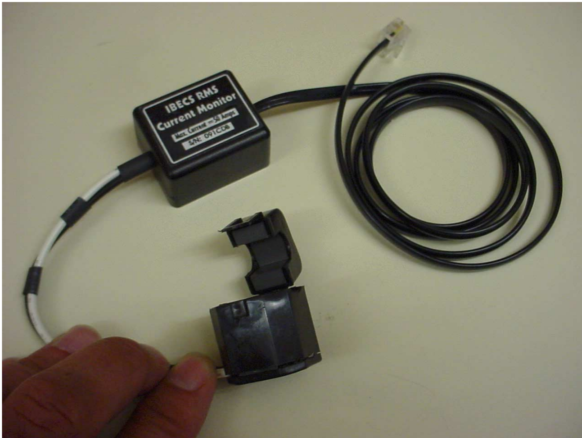
Figure 5. Prototype RMS Current Monitor showing split-core transformer opened for illustrative purposes. In a real installation, the conductor carrying the current to be measured is placed in the transformer and the cover snapped shut. The black cable is standard Telco cable (4 conductor, RJ-11 terminator) and plugs into an IBECS network.
