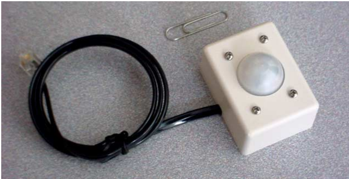
Figure 1. Prototype workstation multisensor designed to measure desktop illuminance, temperature and occupancy. This workspace multisensor measures the three key environmental variables and outputs this digital data onto the IBECS network. The Multisensor is designed to be mounted near the primary work area and plugs into a port adaptor that is attached to the serial port on the user's PC.
