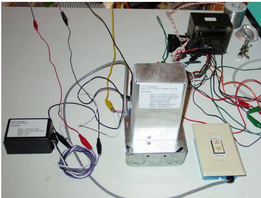
Figure 9. Photo of the Phase Cut Carrier Decoder, Encoder and wallbox control unit (shown from left to right) before shipping to PG&E's Thermal Testing Facility for reliability testing.
