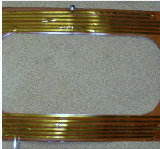
Stainless steel tape heaters between coils for energy deposition experiments
