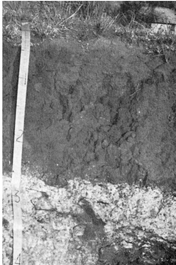
Figure 4.—Profile of an Acuff loam. The layer of calcium carbonate accumulation begins at a depth of about 36 inches.
