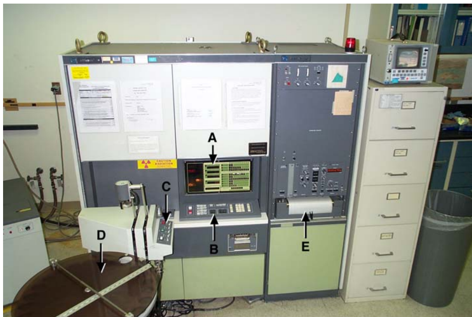
Figure 4. The XRF instrument at LANL. A) Panel for display of elements currently being analyzed and their count rates, B) Operation control panel, C) Control panel for sample changer, D) Automatic sample changer, E) Chart recorder for wavelength scans of X-ray intensities.
