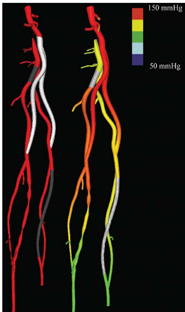
Figure 2: Looking at the options presented by the ASPIRE System, doctors can see which treatments will produce acceptable pressure drops in patients, guiding their decision for treatment type. The pressure map offers a quick way to evaluate pressure losses associated with each treatment. Here, two treatment options are provided; the pressure distribution (generated using finite element methods) is captured during peak systole for a pre-operative case of ilio-occlusive disease, or complete closure of the air passage. The gray bands represent a complete blockage of the artery due to plaque formation. Graft implant: end-to-end aorto-iliac bypass.
