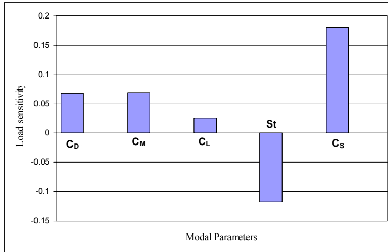
Figure 6.14: Sensitivity of the maximum load to the variation in model parameters for design spar in 3,000 feet of water under hurricane loading
