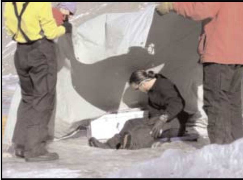
At left, John Priscu's limnology team works in an orange fabric shelter on Lake Hoare to protect microbial life in the water samples they are taking from being shocked by the light. Jill Mikucki fills labeled bottles with water drawn up from a specific depth with a handcrank while Tucker Stevens looks on. Nutrients are added to some of the sample bottles, which are then suspended on a line back under the ice to see how the added nutrients affect their productivity. To lower the samples into the ice without exposing them to light, Brent Christner is covered with a tarp, above. The samples will be analyzed both in Antarctica and back at Montana State University in Bozeman.
