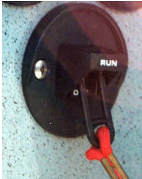
Figure 9. Kill switch with lanyard attached.
