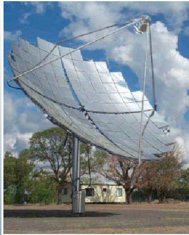
Point Focus Reflector and its 20kW Receiver
