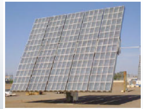
25 kW Point Focus Fresnel Lens
