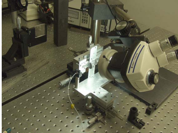
Figure 7. Set-up for exposing fiber to excimer laser output.
