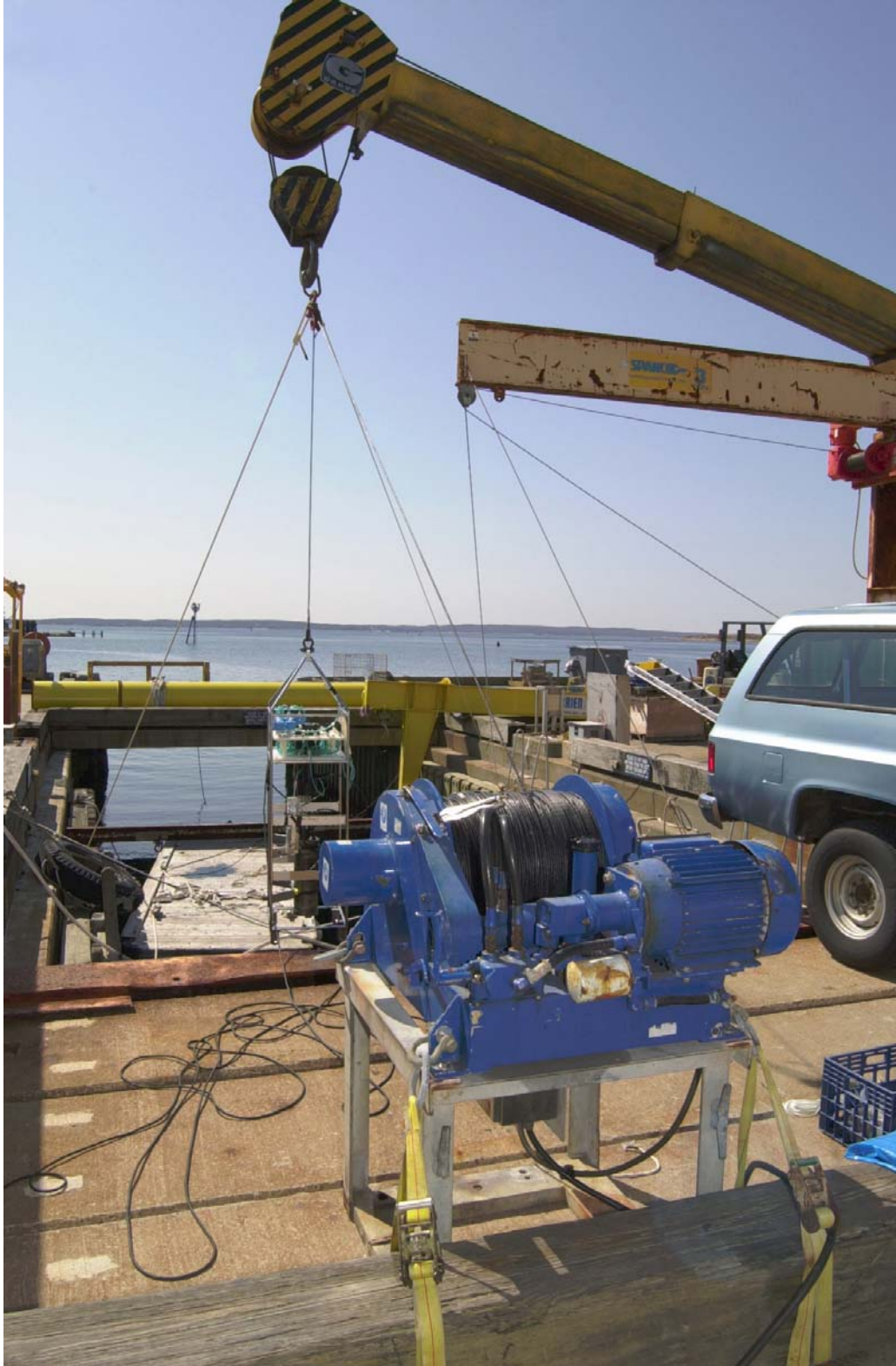
Figure 6. Configuration of equipment used to lower the WTS-Tr instrument into the water during a field test at the Woods Hole Oceanographic Institution (WHOI) dock facility.
