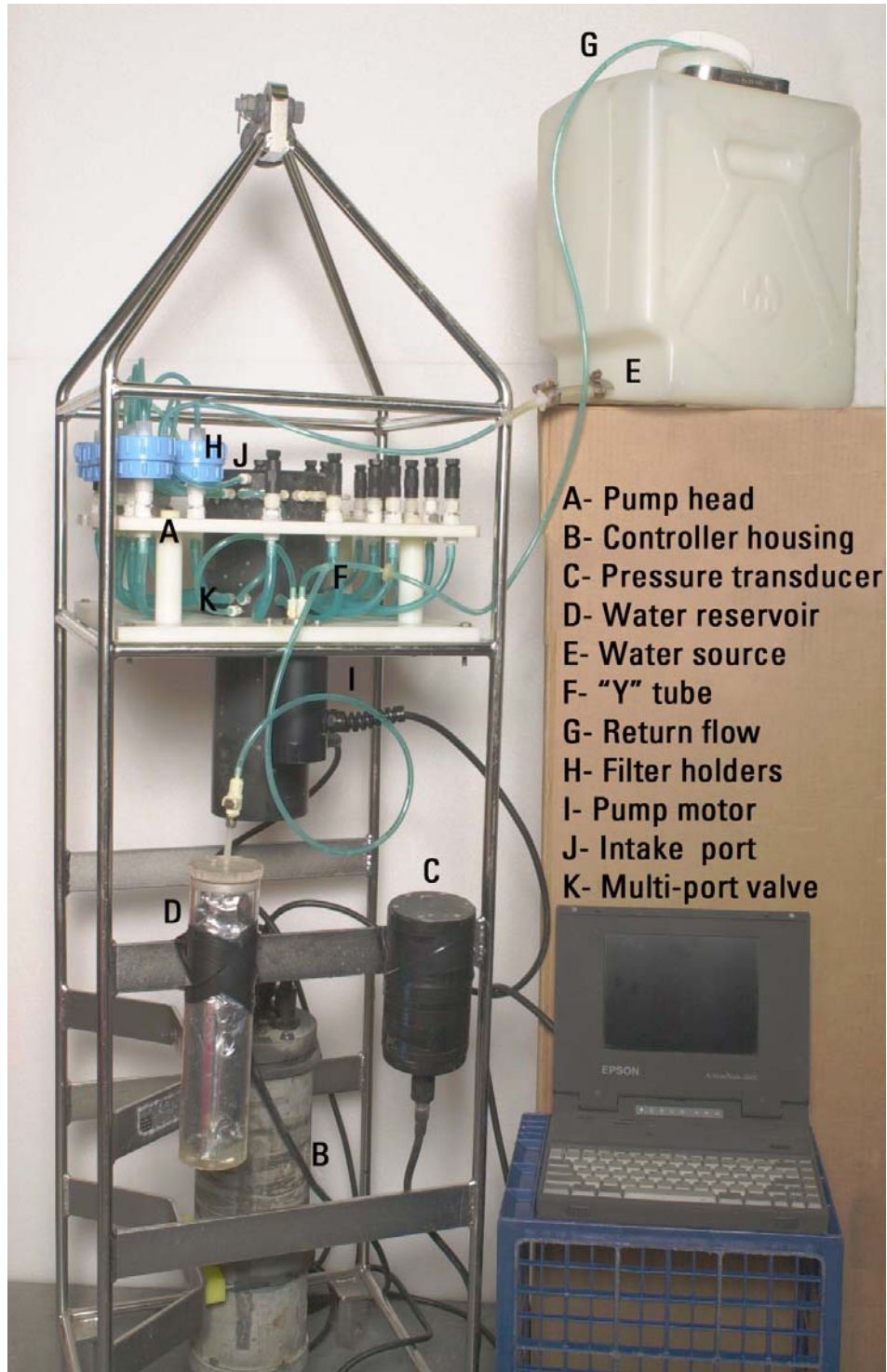
Figure 1 B. The Mclane WTS WTS-P suspended sediment sampler showing the overall system and configuration during laboratory testing procedures.
