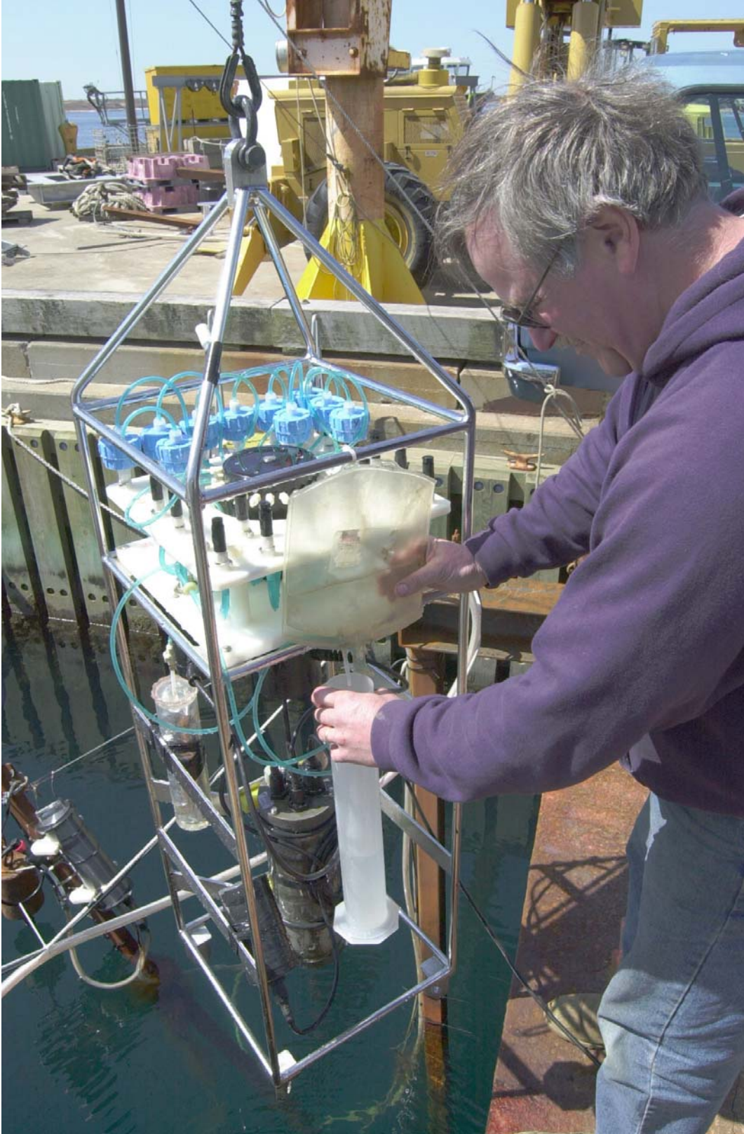
Figure 7. Collection and volume measurements of water pumped through the WTS-Tr system during testing procedures at the WHOI dock facility.
