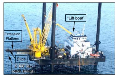
Figure 2: Lift boat, extension platform
