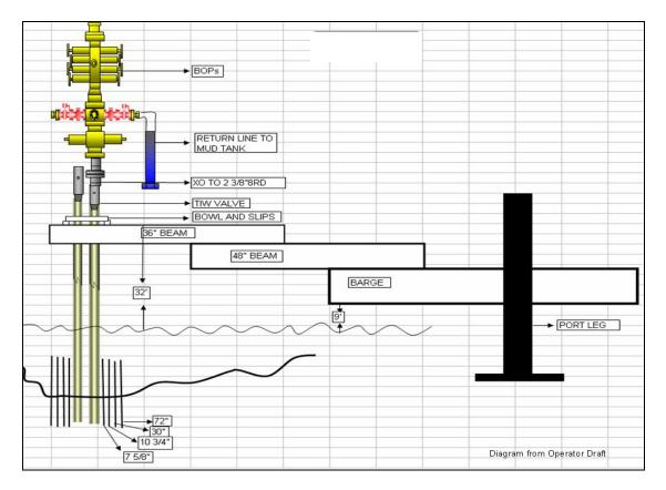
Figure 6: Diagram of lift boat, tie-back tubing, well head
