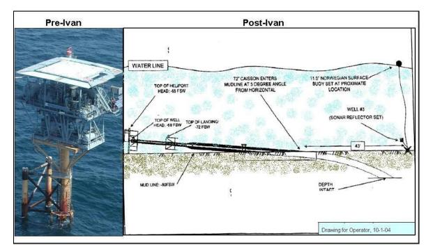
Figure 5: Main Pass 98, Well # 3 caisson, pre-Ivan, post-Ivan
