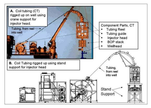
Figure 10: Coil tubing unit components
