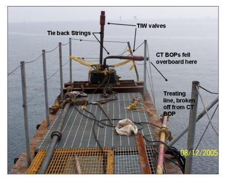
Figure 9: Extension platform after accident
