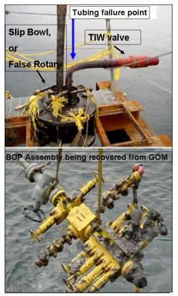
Figure 3: False rotary or slip bowl and BOP assembly
