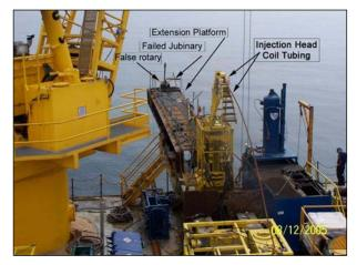
Figure 7: Extension platform, CTU injection head
