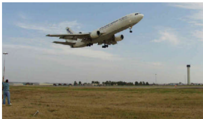
The FedEx MD-10 completing a LAAS Test Prototype guided approach to runway 18R at Memphis International Airport. The pseudolite antenna appears on the left side of the picture.
