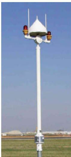
LAAS Test Prototype reference stations installed at Memphis.
