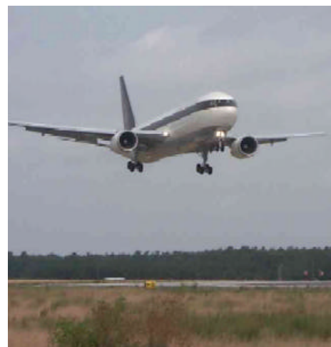
UPS B767 completing a LAAS Test Prototype guided approach to runway 13 at Atlantic City International Airport.
