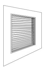
An exterior shade screen fits neatly within window framing, a bit away from the glass. Design for easy removal for cleaning.
