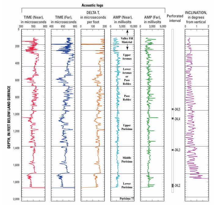
Figure 6. Acoustic and borehole inclinometer geophysical logs for the deep-aquifer system monitoring-well site, Marina, California.
