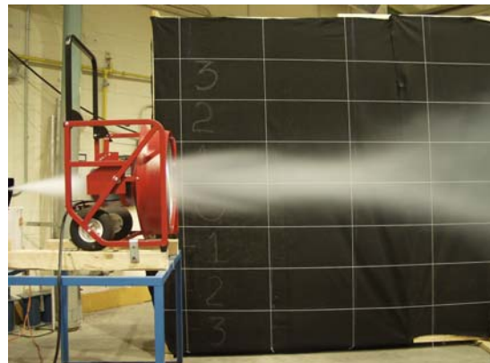
Figure 10. Layout for phase I flow visualization experiment.
