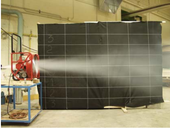
Figure 11. Visualization of PPV flow.
