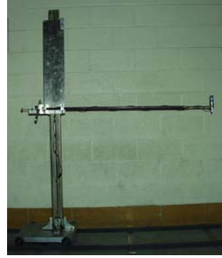
Figure 6. Anemometer in indexer on track.
