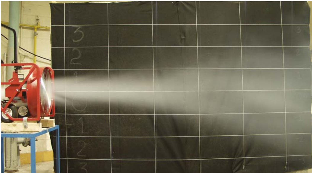
Figure 41. Experimental visualization of the PPV flow pattern.
