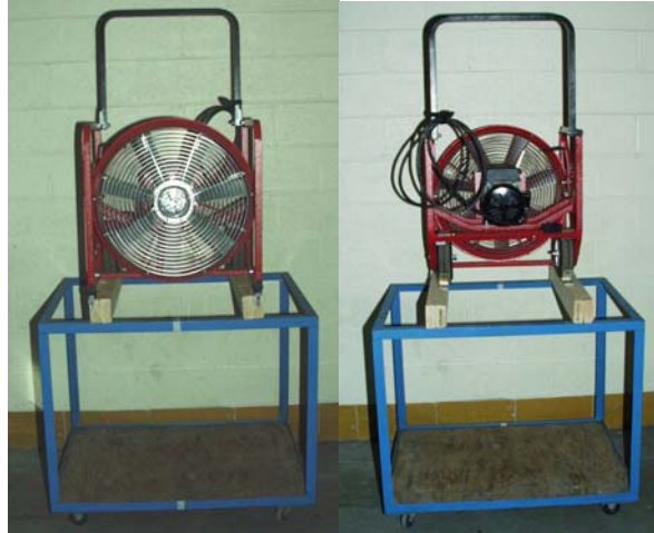
Figure 4. Front and back of the positive pressure fan and stand.
