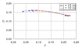
Fig. 7. Duct extension effect on thrust coefficient, axial flow conditions.
