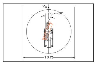
b) Forward flight orientation,  $\alpha = 0 \text{ deg } (\alpha = -20 \text{ deg indicates orientation of duct, not support structure})$
