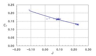
a) Thrust coefficient, shaft axis
