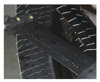
Fig. 3. Exit vane with 1-in flap
