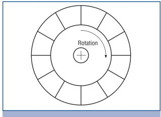
Figure 2-3. Radial-Blade Centrifugal Fan
