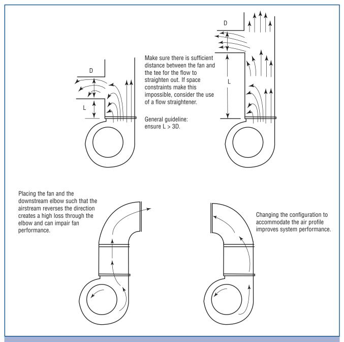
Figure 2-18. Fan Outlet Conditions
