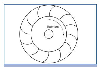
Figure 2-1. Forward-Curved Blade Fan
