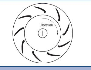
Figure 2-7. Backward-Inclined Centrifugal Airfoil Fan
