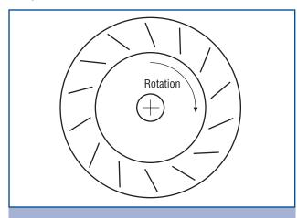
Figure 2-6. Backward-Inclined Fan
