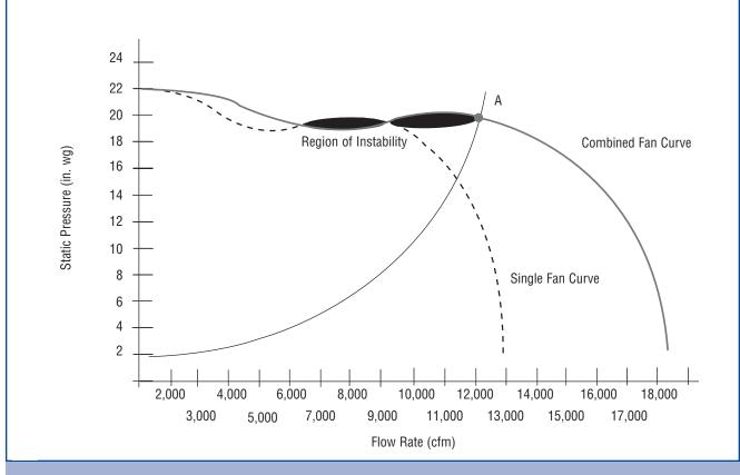
Figure 2-25. Instability Region Because of Parallel Operation of Identical Fans
