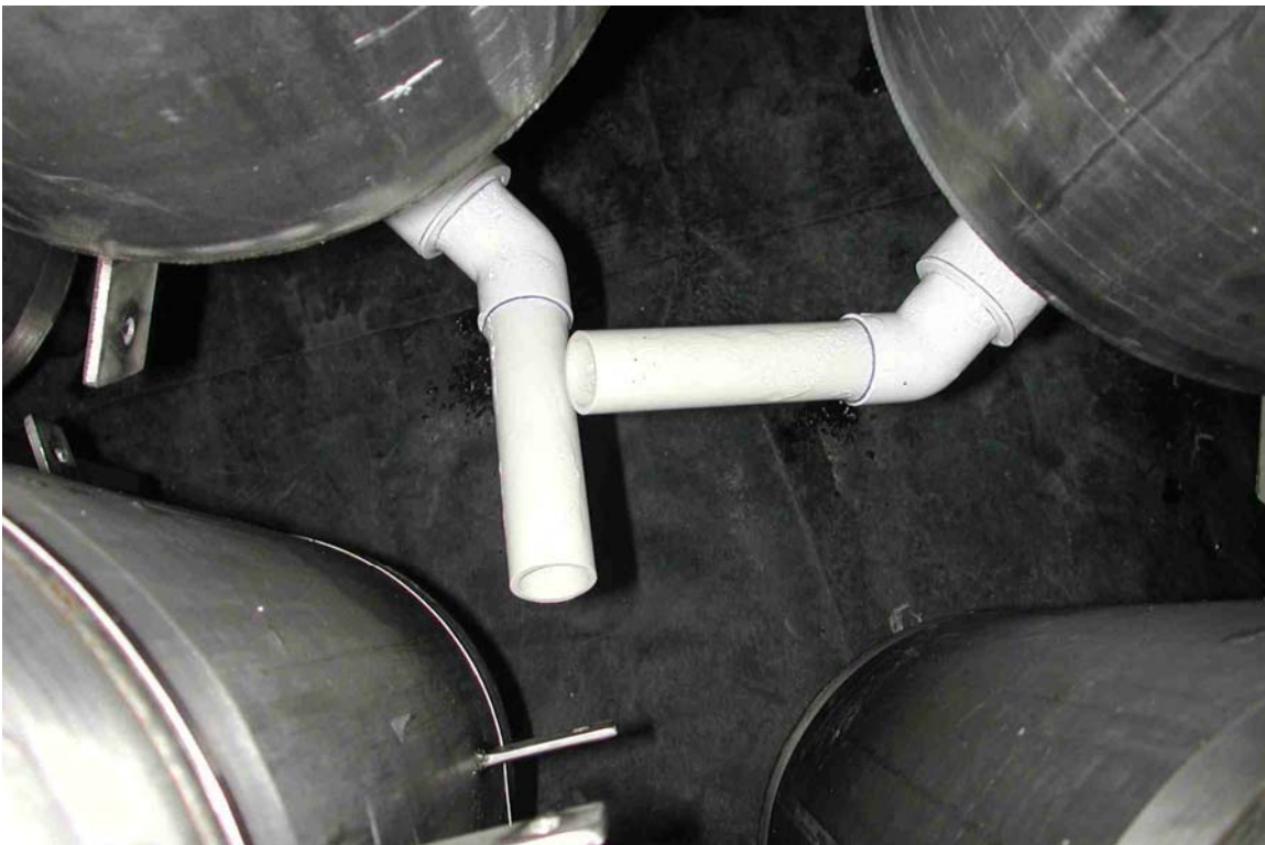
Figure 2.7. Final Prototype LS PVC Nozzle Relationship
