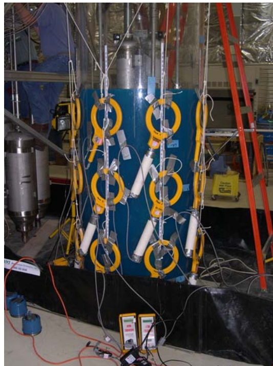
Figure 5.7. Antenna Placement for Laponite Test (similar to configuration used in slurry tests)
