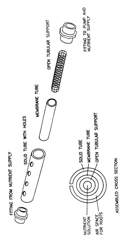
Figure 1. Schematic diagram of the Tubular Membrane Plant Growth Unit used in the wheat trial.
