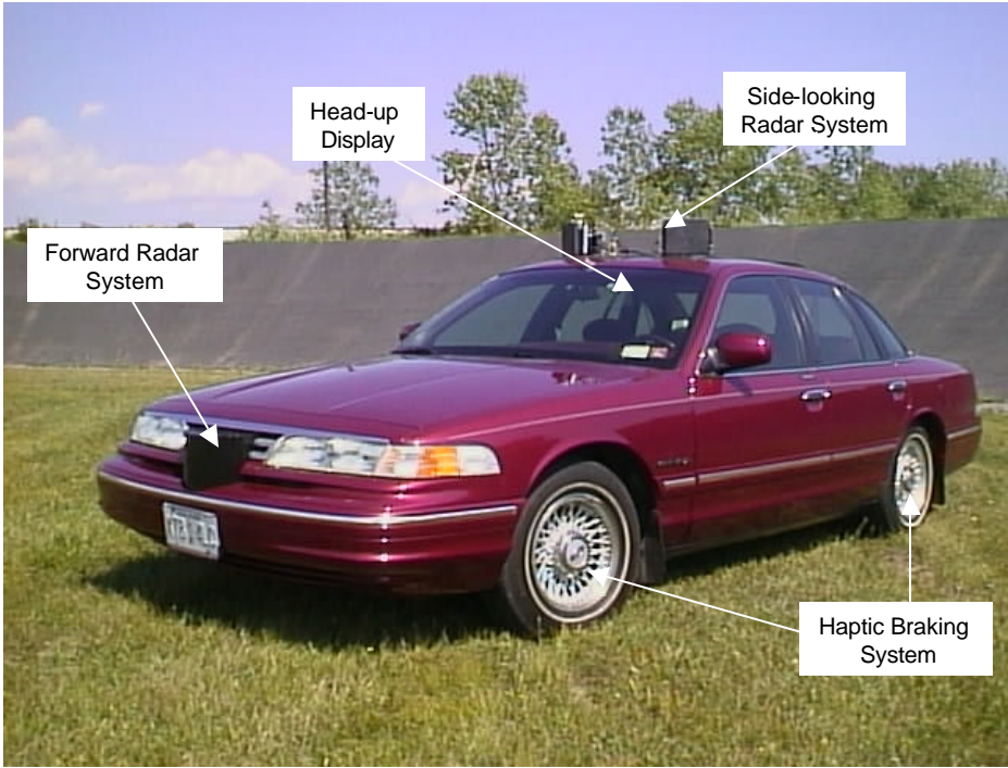
Figure 4-2 The ICAS Testbed
