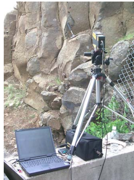
Figure 1.—Portable laser vibrometer, dynamic signal analyzer, battery pack, and data collection computer.
