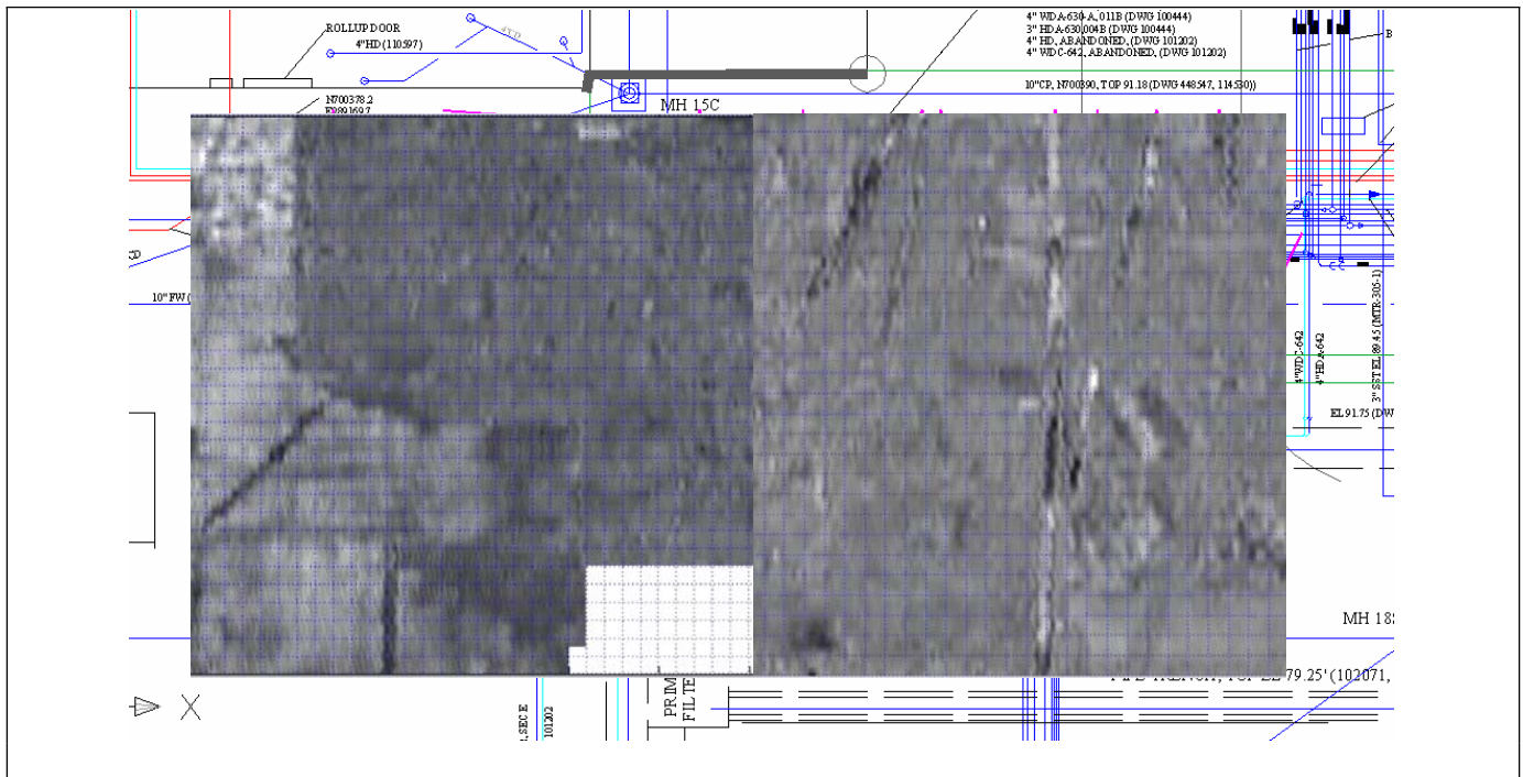
Figure 4: GPR time slice data from a recent utility project. This data represents an area approximately 60 meters by 30 meters. The GPR data was collected in two overlapping sections (5 meter overlap) to allow for smaller data sizes and to ease interpretation. Interpretation is problematic for data sets greater than about 15 to 20 meters on a side and these data sets were further divided for interpretation. This study found some utilities that seem to correspond to major utility corridors in the map, but many of the utilities inferred from the geophysical data are shallower than those shown on the map (Figure 6).
