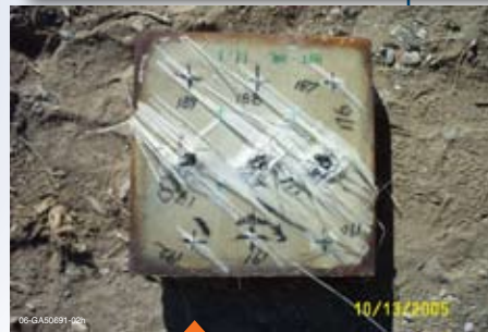
The images above display the results of several high-caliber impacts on two armor samples under evaluation at INL.
