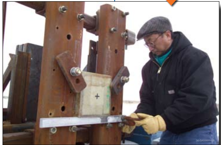
INL researcher Dr. Henry Chu prepares an armor sample for ballistic testing at the laboratories armor penetration test bed.
