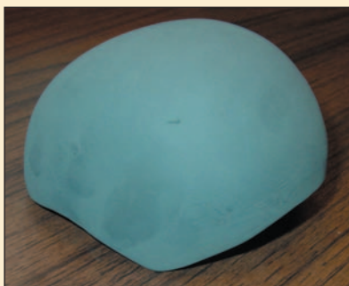
Pressureless sintering allows fabricating complicated, curved shapes for use in helmets and other body armor. Here, a small-scale prototype helmet is shown.
