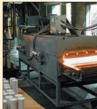
Rapid heating of forging tooling using infrared heating.
