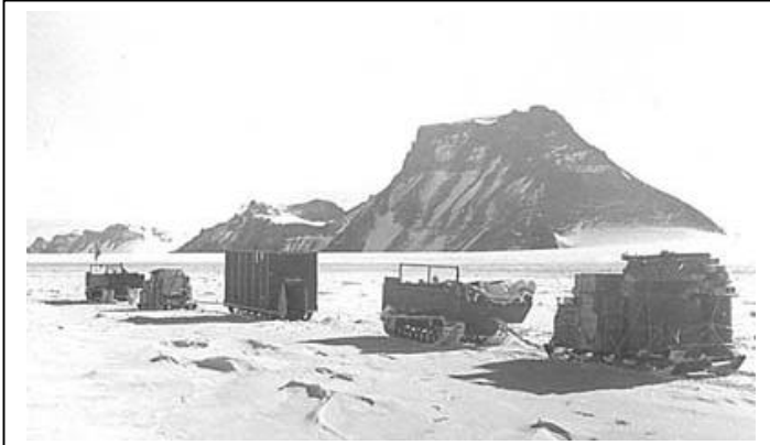
Figure A.8 A seismicology traverse. The lead Weasel tows a supply sledge and a mobile shelter for the seismic equipment. The trailing Weasel tows a heavily laden supply sledge.
