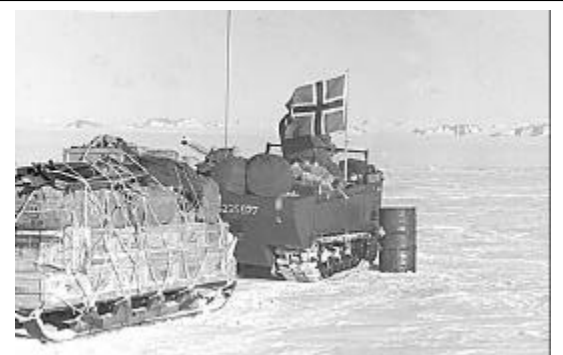
Figure A.3 “Weasels” -- amphibious tracked vehicles developed by the U.S. Army in World War II -- were used to transport people and tow sledges loaded with supplies.
