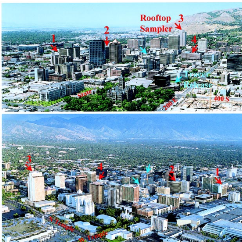
FIG. 7. Downtown SLC showing the four elevated tracer sampler locations (red arrows) and two downtown tracer release locations (blue arrows). The top picture is looking to the northwest and the bottom picture is looking to the southeast. (Photographs from Don Green Photography, Salt Lake City, Utah.)
