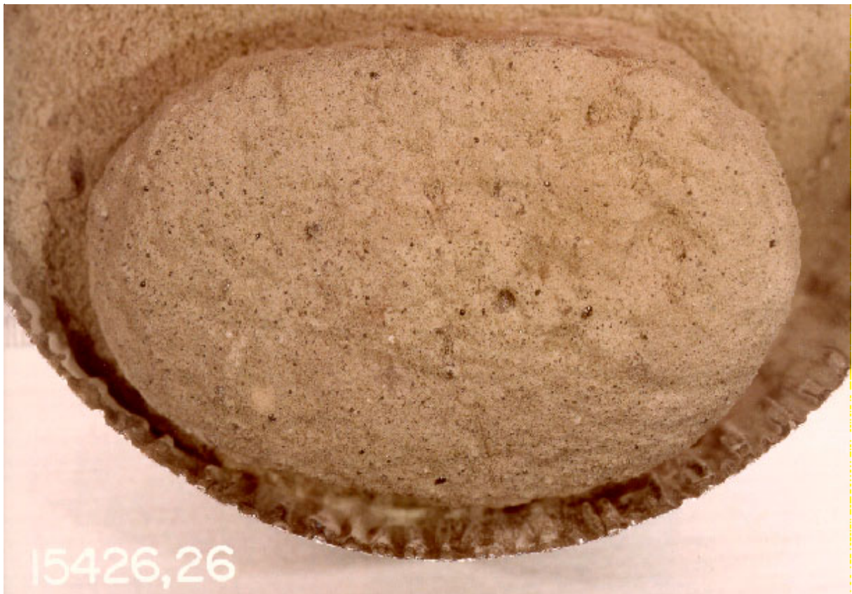
Figure 3: Close up of 15426,26 showing that glass beads are only about ~5 % of rock, with the rest of very-fine off-white powdery material. Sample about 3 cm across. NASA S80-42656.
