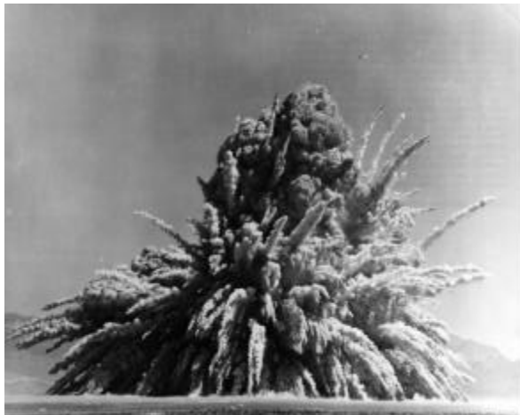
Plumes of sand and dust formed by boulders and clumps of gravel ejected from the desert by the July 6, 1962, Sedan Plowshare test. Source: REECO, Bechtel Nevada.
