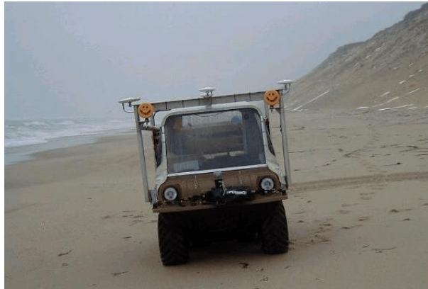
Figure 4: SWASH. Note the multiple GPS receivers on the top of the buggy.
