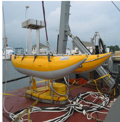
Figure 3: The new seismic reflection system with the “cataraft” sled designed at the Menlo Park Center so data can be collected in water <10 m deep.
