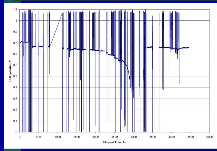
•101 Thermal Cycles •-0.78%/1000hr overall degradation •Consistent **OCP** through test •3073 hours operation •Cycling continues
