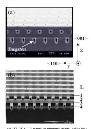
IMAGES OF A 3-D tungsten photonic crystal, taken by a scanning electron microscope. The images taken with and without oxide are shown in (a) and (b), respectively. The 1-D tungsten rod-width is 1.2 mm, the rod-to-rod spacing is 4.2 mm, and the filling fraction of tungsten material is 28 percent. The spacing of the rods acts to transmit certain frequencies of light. The structures show great promise for converting heat to light.
