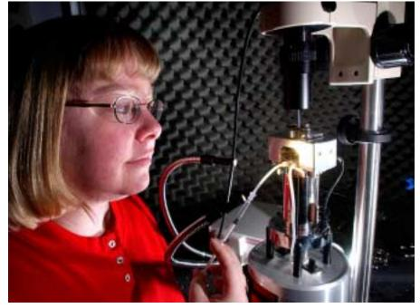
TRACKING RECEPTORS — Sandia postdoc Julie Last (1140) uses an atomic force microscope to image the travels of receptor-lipids on an artificial cell membrane.
