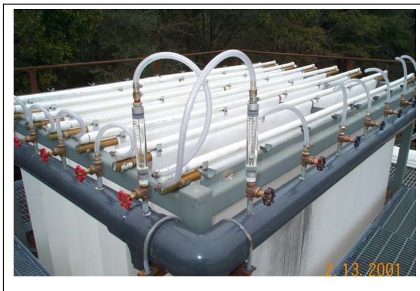
Figure 3. Top View of Water Distribution Test Stand
