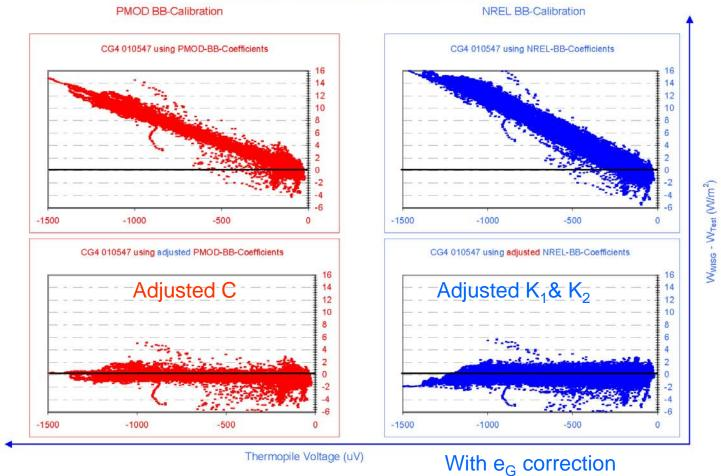
Difference between the reference irradiance (WISG) and the irradiance measured by the test pyrgeometer at PMOD/WRC between July and December 2007.
