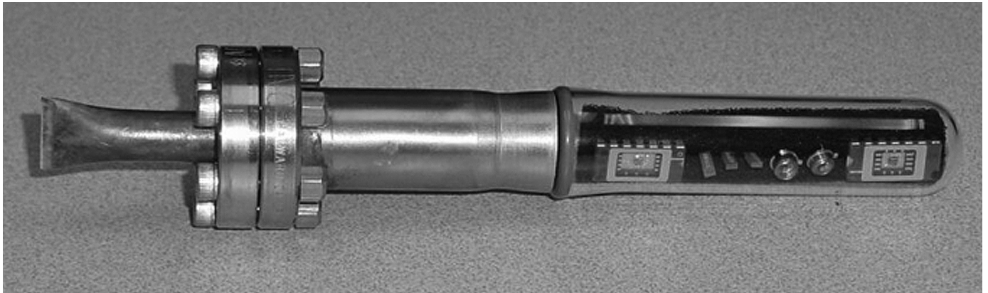
Fig. 1. Picture of parts mounted in glass tube with 100% H 2 .
