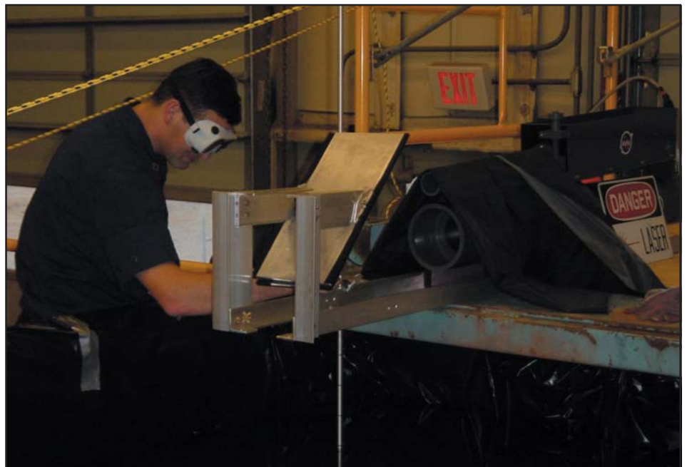
Top: Representatives from Laser Diagnostics Instruments International, Inc. (LDI3) prepare to test their Light Detection Ranging systems (LIDAR) in a test tank
