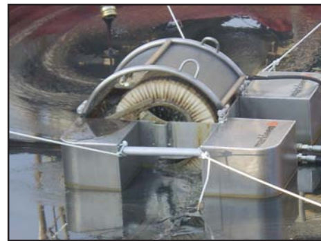
The Quali Tech Environmental stationary skimmer being tested to determine its maximum oil recovery rates and corresponding oil recovery efficiencies
