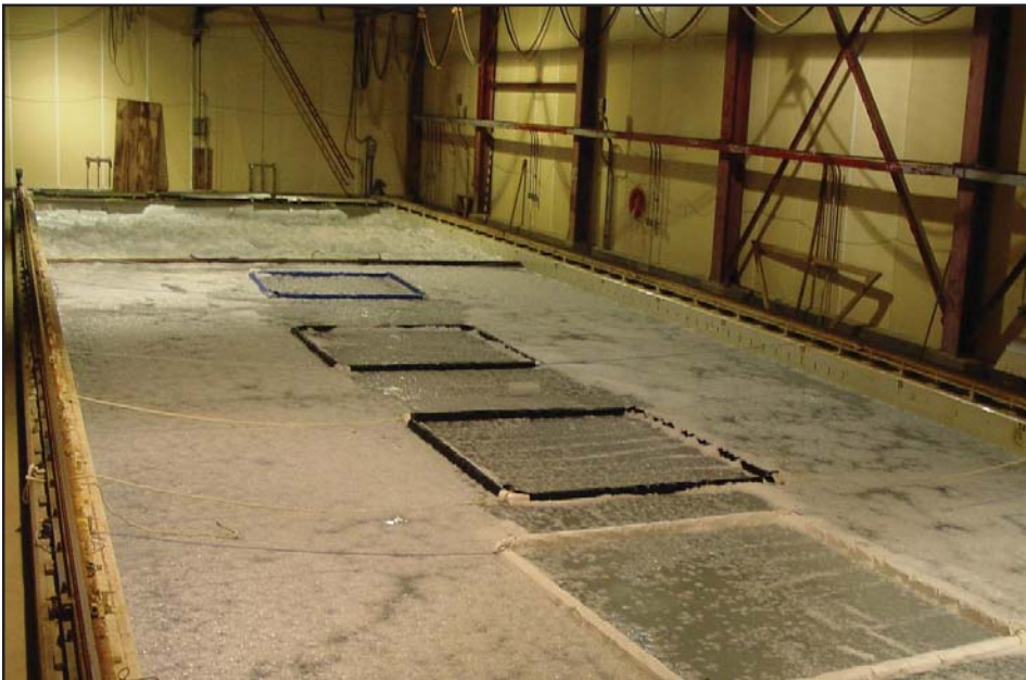
Seven skirted boom test frames were injected with oil, then frozen in place at the CRREL facility in New Hampshire
