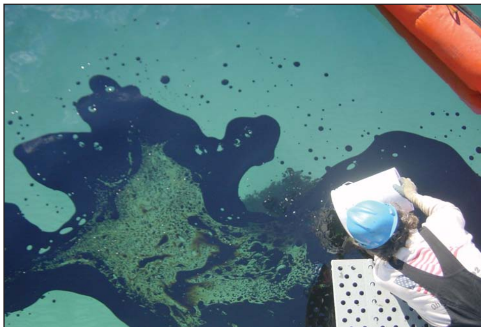
An Ohmsett technician places oil on the tank water during a study to determine what emulsions created at sea might look like based on emulsions created in the test basin
