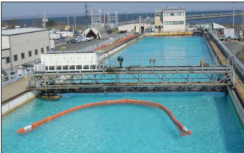
The NOFI Trömsö prototype boom system's performance is put to the test
