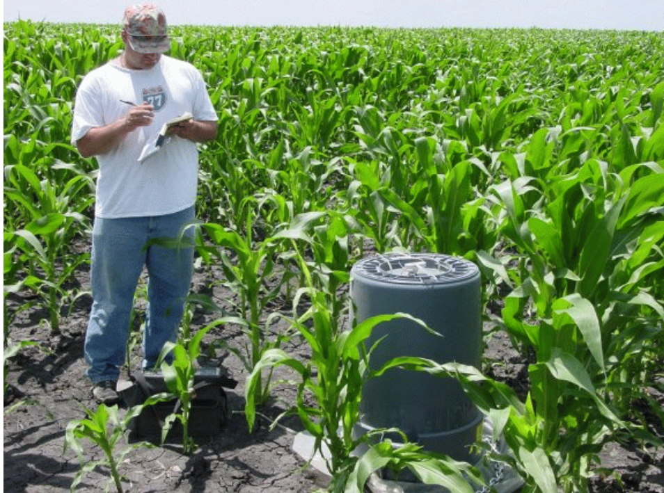
Large skirted chamber used for CO 2 flux from corn/soil system. Applicability of chamber for N 2 O and CH 4 flux measurements has not been tested.
