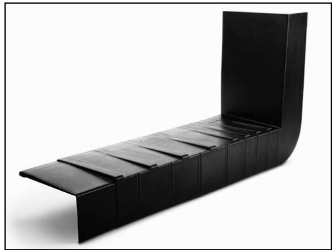
Figure 11. The Marvin SillGuard (above) is far more rugged than the Dow sill pan. The flashing is sloped to the exterior; integral ridges keep the window frame above the drainage plane.
