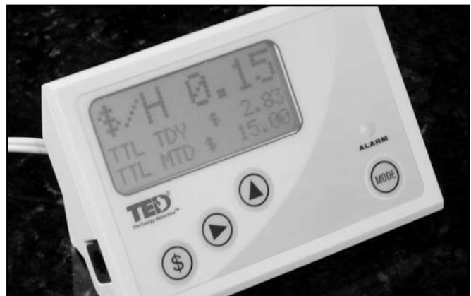
Figure 8. The Energy Detective’s display unit can be plugged into any convenient electrical receptacle.
