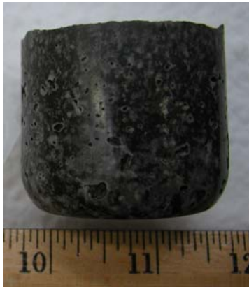
Figure 3.9. Portland Type III Grout Monolith
