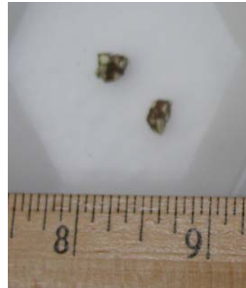
Figure 3.10. Grouted AgZ + CaI 2 Sized for TCLP Testing
