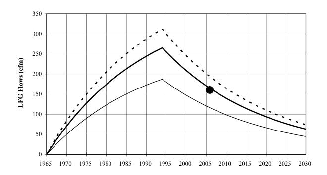
**LFG Generation** LFG Recovery at 85% Collection Efficiency LFG Recovery at 60% Collection Efficiency **Actual LFG Recovery in July 2005**
